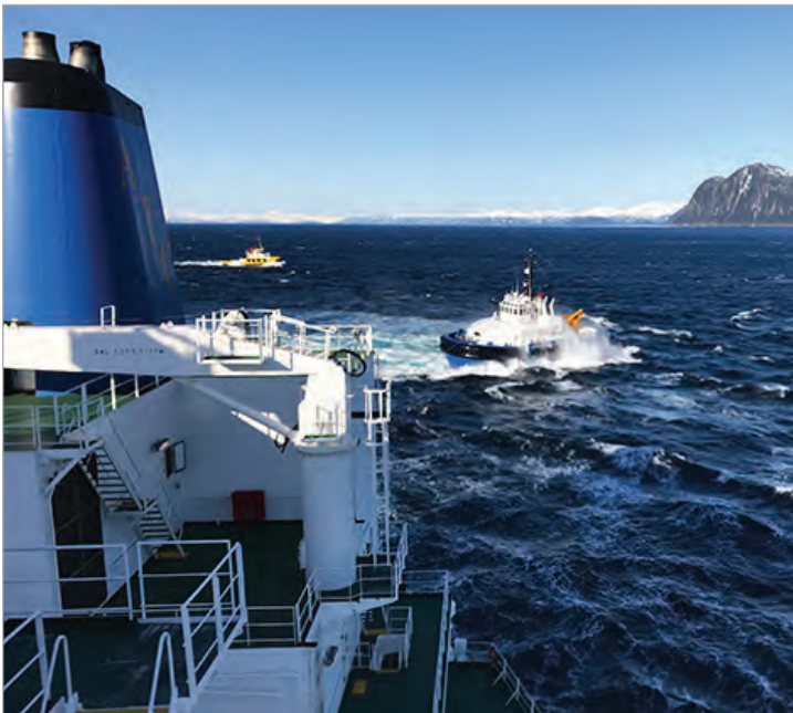
Tether drill: Alyeska and ECO have conducted more than 60 tether and towing exercises with tankers since the vessels started arriving in March. Above, the Commander maneuvers during a tether drill.
