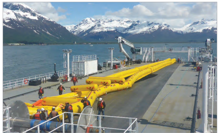
The decks of the new oil spill response barges are large enough to completely inflate the new Current Buster 8 oil spill boom on board, rather than partially inflating in the water. The new method is easier and safer for the crews.
