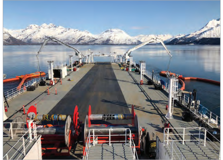
Barge deployments: Alyeska and Edison Chouest have bi-weekly barge deployments so that crews can practice and demonstrate their proficiency operating the new skimmers and boom aboard the purpose-built barges.
