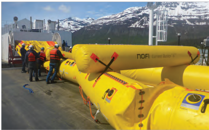
The decks of the new oil spill response barges are large enough to completely inflate the new Current Buster 8 oil spill boom on board, rather than partially inflating in the water. The new method is easier and safer for the crews.
